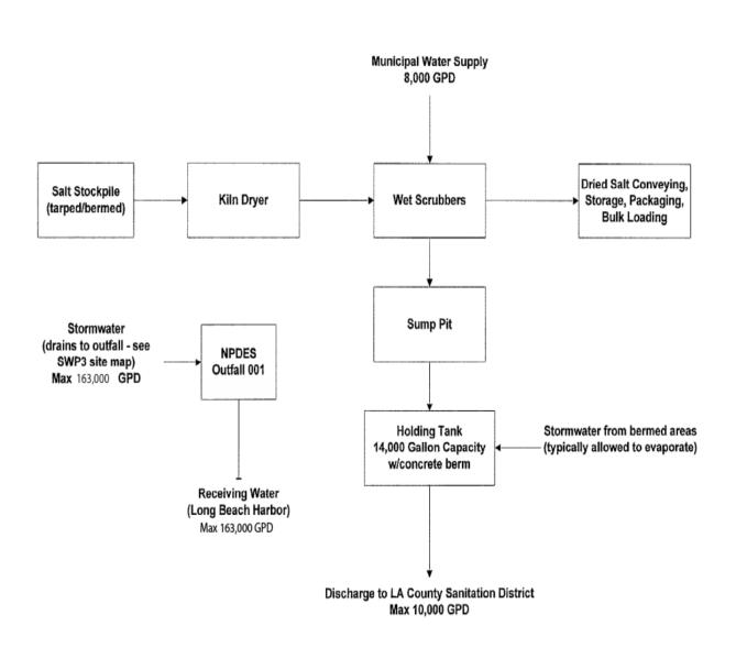
Line Drawing - Morton Salt, Long Beach Facility (Wastewater Flow)
