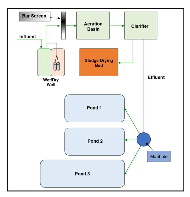
ATTACHMENT C - PROCESS FLOW DIAGRAM
