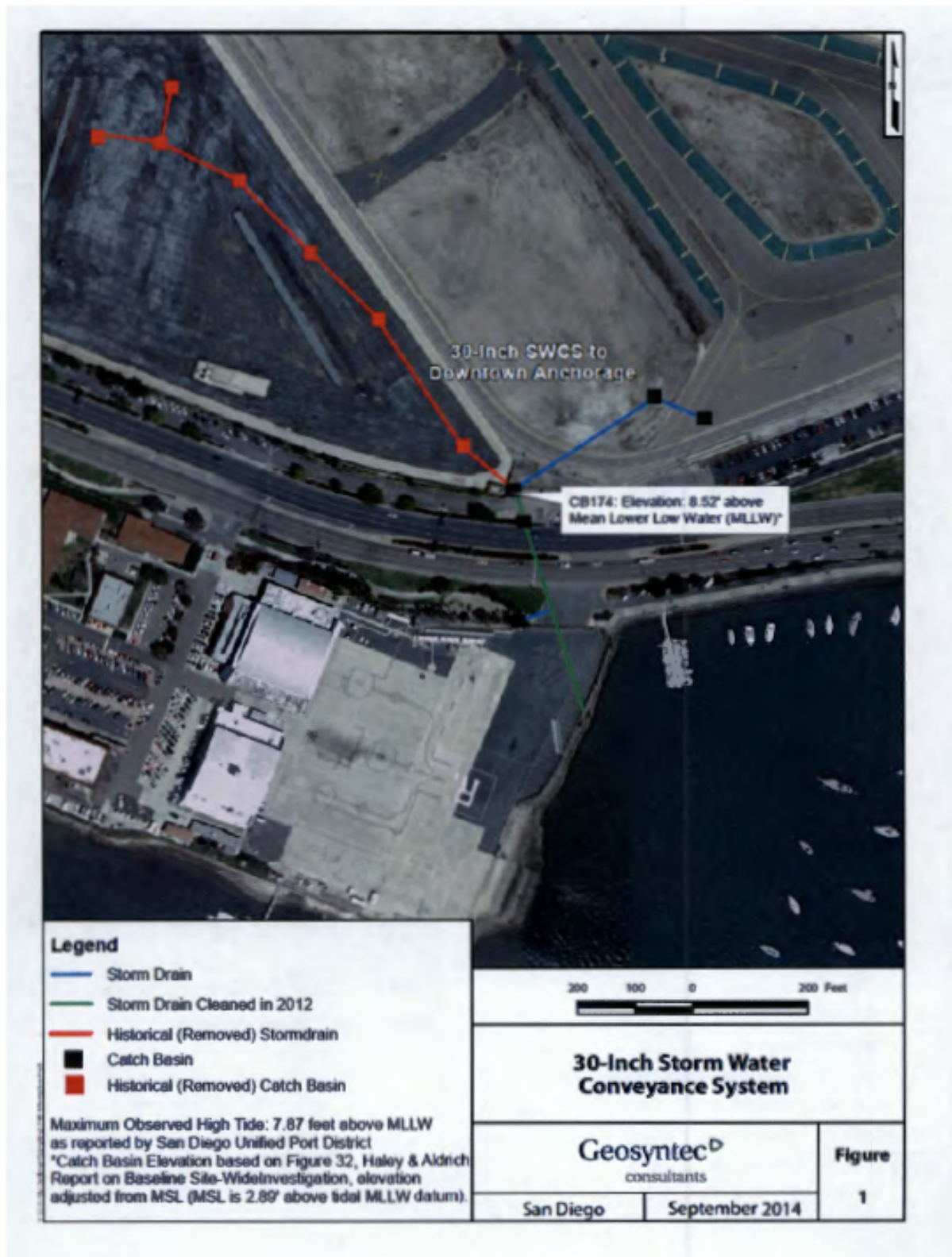
Figure 1 30 Inch Storm Water Conveyance System
