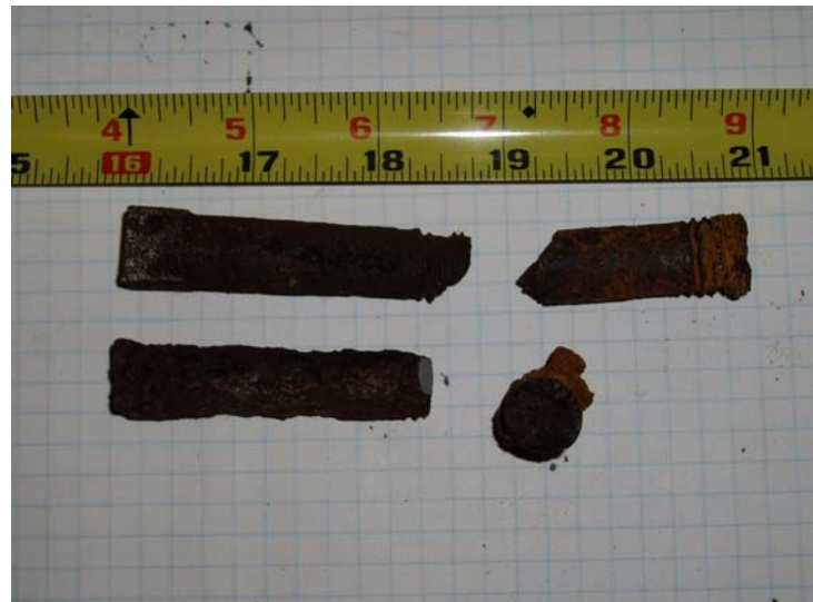
Figure 14 – Corrosion of fasteners
