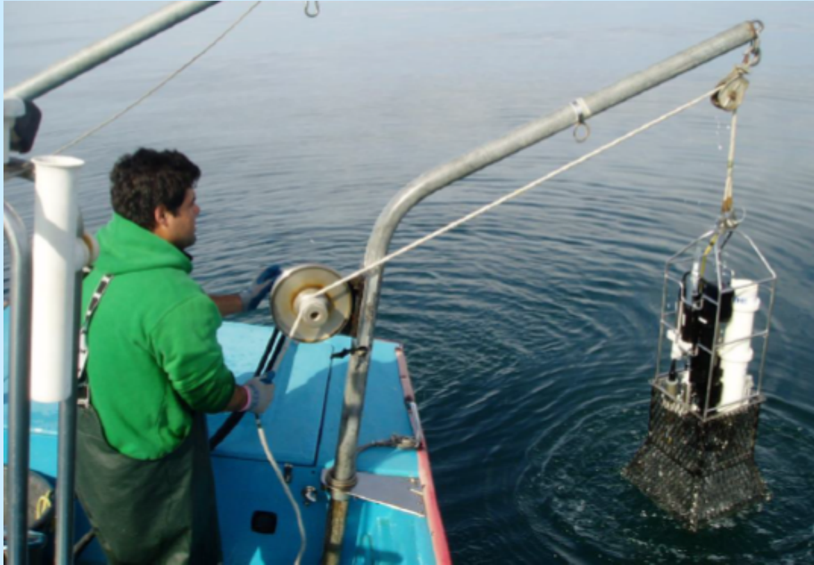
CTD = Conductivity, Temperature, Depth Sensor
