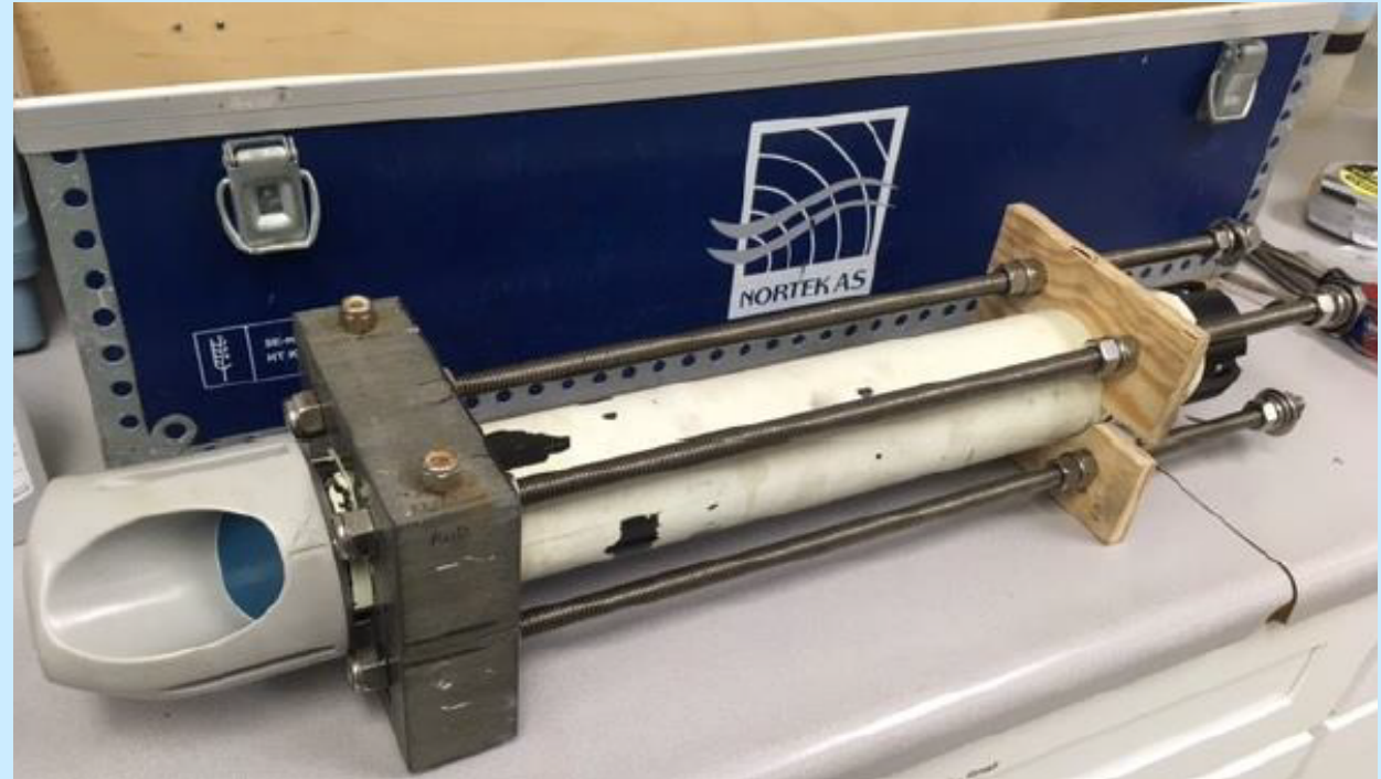
ADCP = Acoustic Doppler Current Profiler
