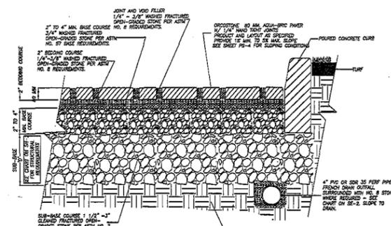
STANDARD INSTALLATION WITH CONCRETE CURB EDGE RESTRAINT
