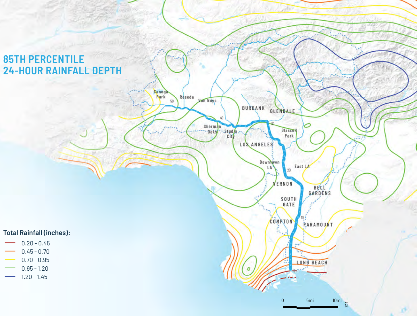
Figure 58. 85th Percentile 24-hour Rainfall Depth. Precipitation in the LA River watershed over 24 hours for an 85th percentile storm. The 1% storm event is approximately an order of magnitude (i.e., 10 times) larger than the typical storm events that are experienced several times per year. Source: Los Angeles County GIS Data Portal, 85th and 95th Percentile Rainfall, 2016, Los Angeles County GIS Data Portal, Rainfall Intensity, 2011; Geosyntec, OLIN, 2019.
