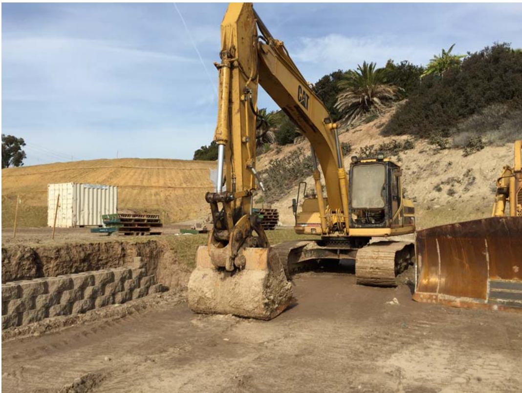
Figure 4. Failure to have vehicle fluid leak protection. Photograph taken by Wayne Chiu, San Diego Water Board on December 15, 2014, of heavy equipment without vehicle fluid leak protection. IMG_5064.jpg
