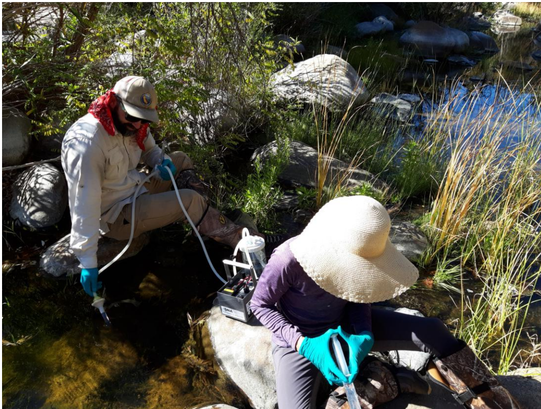
Figure 4. Example collection of eDNA samples using a Smith-Root pump (left) and syringe filter kit (right).
