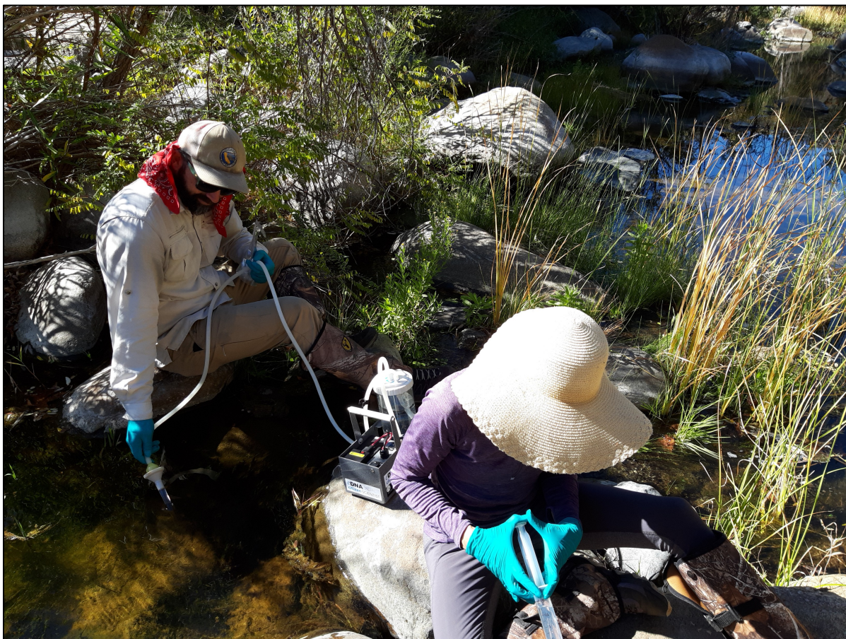
Figure 3. Collection of eDNA samples using a Smith-Root pump (left) and Jonah Ventures kit (right). Water was also collected for vacuum filtration in the lab.
