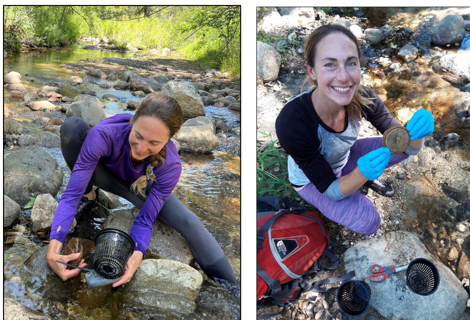
Figure 4. SPATT sampler deployment (left) and retrieval (right). To deploy, a SPATT sampler was sandwiched between two slotted mesh pots and zip tied to a scuba weight.
