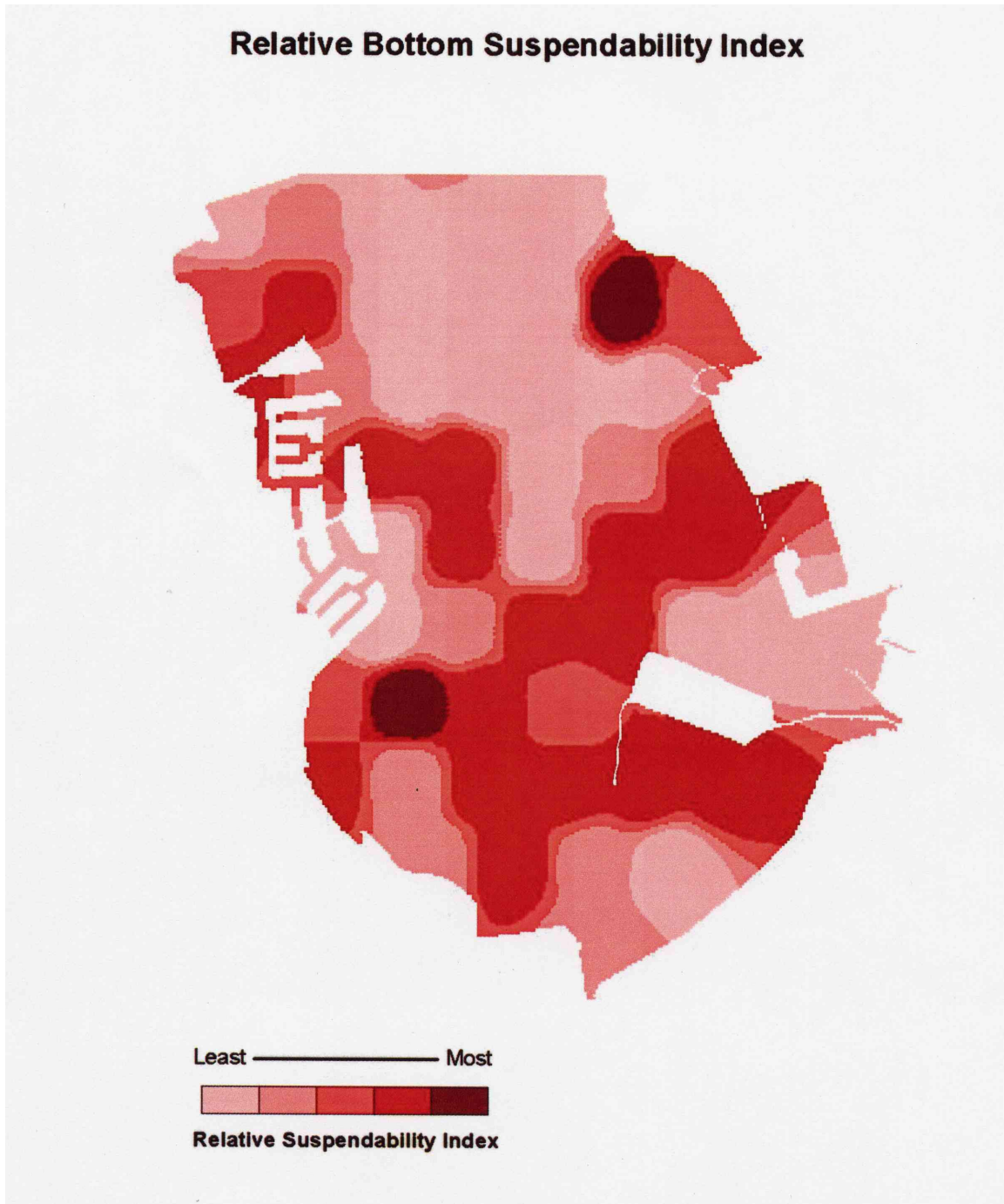
Figure 2.6-19. Relative bottom suspensibility index applied to bottom sediments in South San Diego Bay. Based on data from Merkel & Associates (2000).
