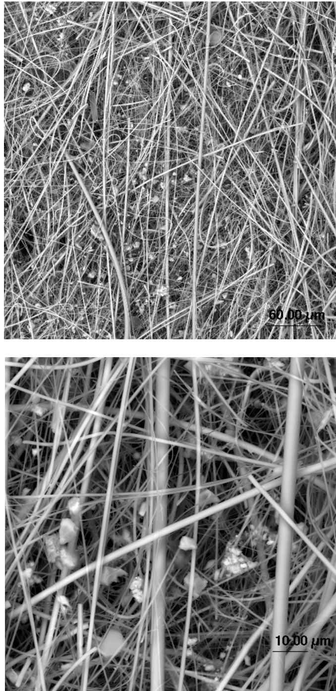
Figure 11. Scanning electron microscope photo of TSS filter used for sand yard discharge water, at two scales.
