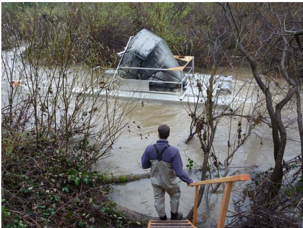
*Rotary Screw trap to monitor fish migrating downstream in the Napa River (Photo Credit: Napa RCD).*
