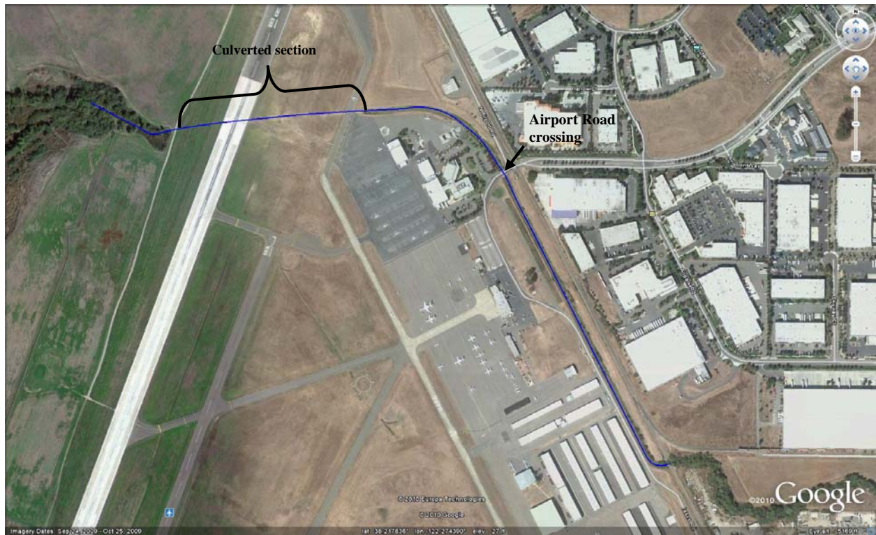
Map A. The upper 3,400 ft of the reach is open channel, which transitions to a 1,350 ft culverted section that flows underneath the airport runway, followed by 600 ft of open channel that discharges to Fagan Slough.
