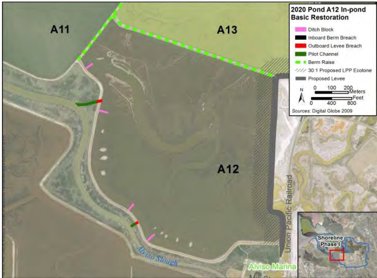
Diagram 2. In-Pond Preparation for Breaching of Pond A12.
