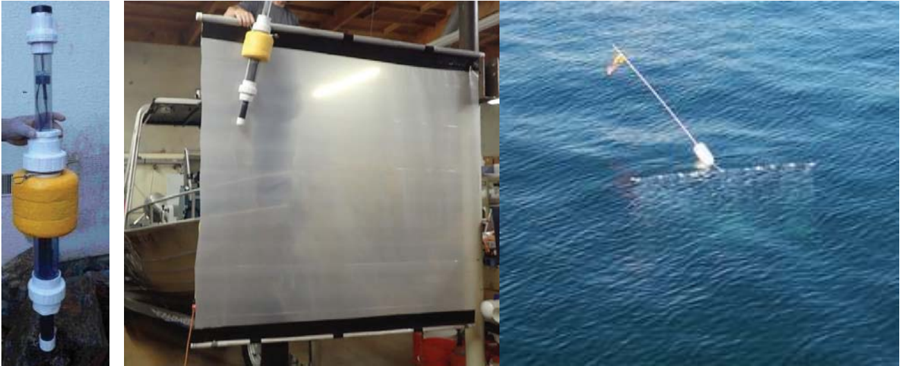
Figure 2-3. Example of current-tracking drogue and GPS buoy
