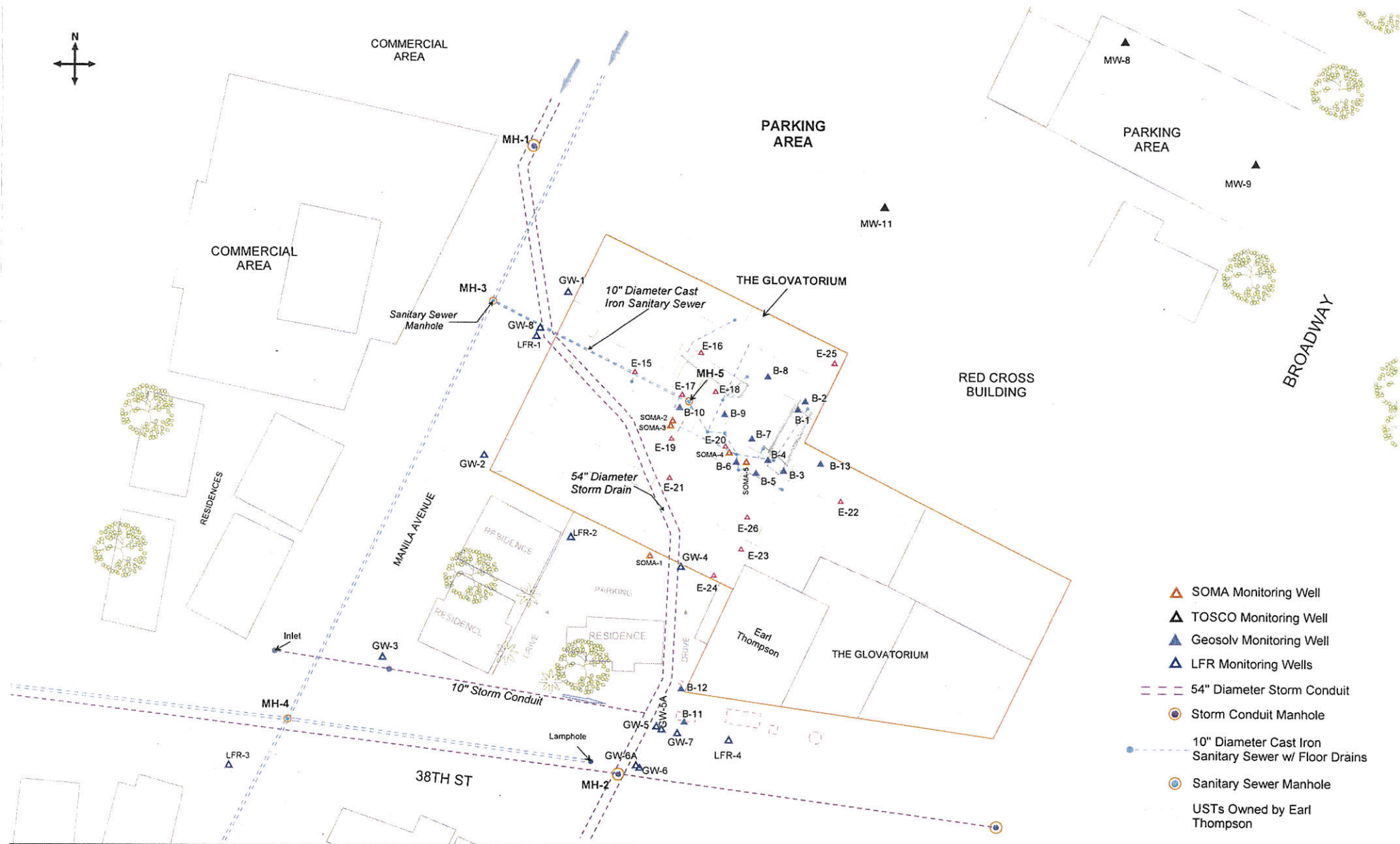
Figure 2: Site map showing locations of monitoring wells, soil borings, and preferential flow pathways.
