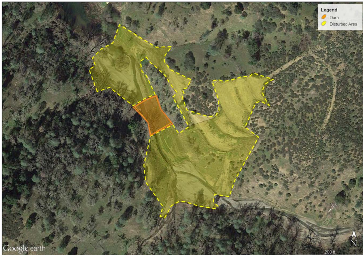
Figure 1. Approximate extent of excavation (dashed area shaded yellow) to generate material for dam construction (solid area shaded orange).
