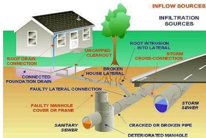
**Figure 9: Sources of Infiltration and Inflow (U.S. EPA Fact Sheet, June 2014)**
