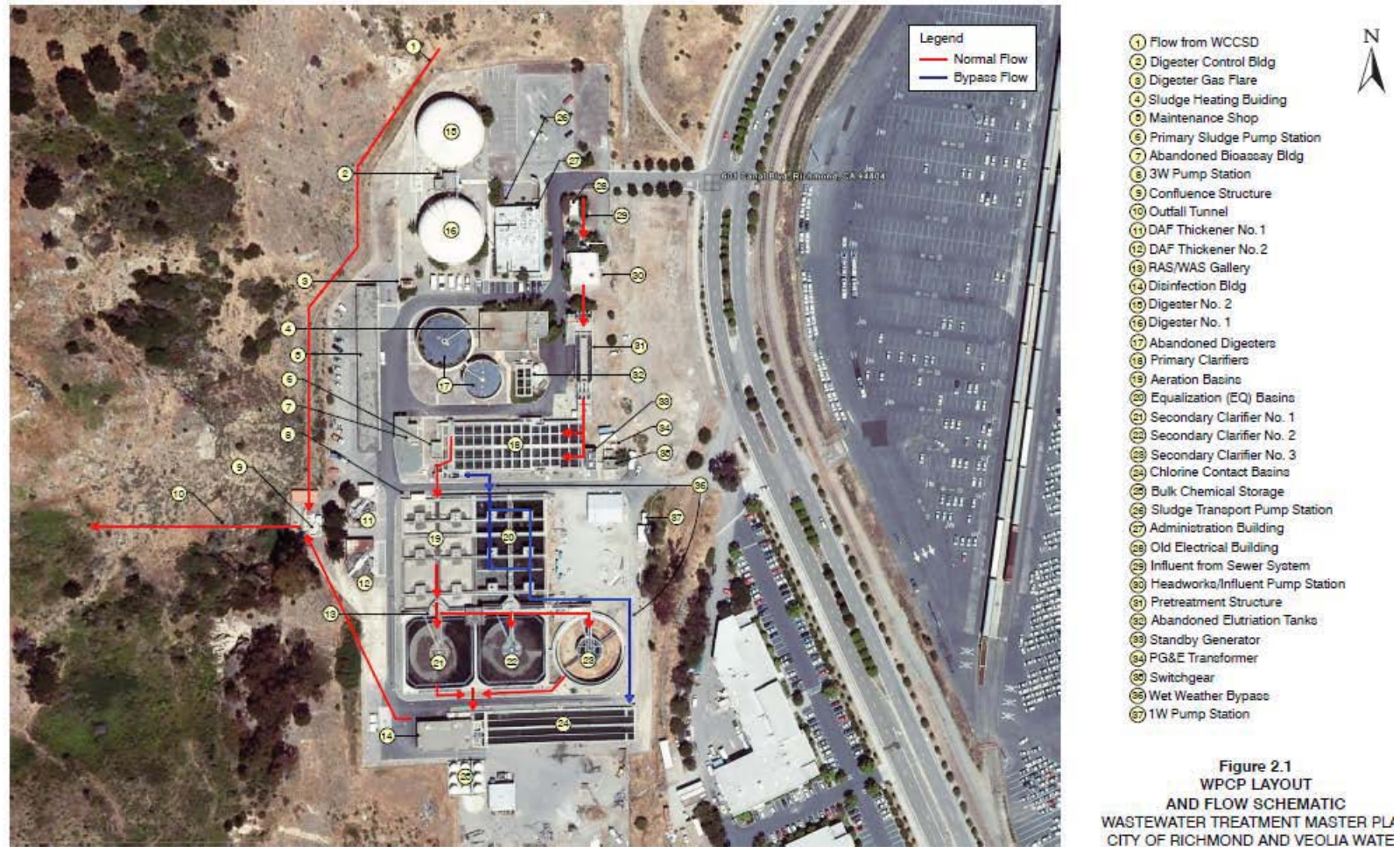
Figure B-3. City of Richmond Municipal Sewer District Water Pollution Control Plant – Layout and Flow Schematic
