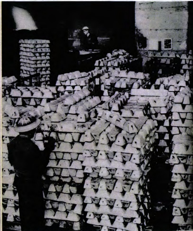
Headaches for Hitler: The camera's eye catches a portion of a day's production stacked in a corner of the ingot handling room of the Permanente foundry. After laboratory analysis, this magnesium will be shipped by boxcar and truck and soon will be transformed into airplane parts or into incendiary bombs. Joe Baltran daubs varicolored spots of paint on the ingots to indicate different types of alloys, as Lawrence Schroyer , jeep operator, warps another stack onto the scale platform.
