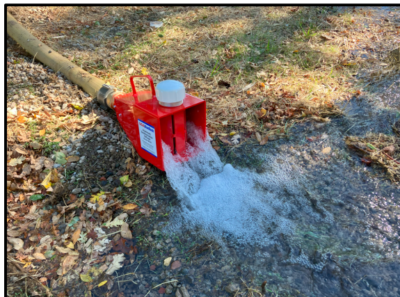
Figure 4: Verano Aquifer Storage and Recovery Well discharge dechlorinator and diffuser
