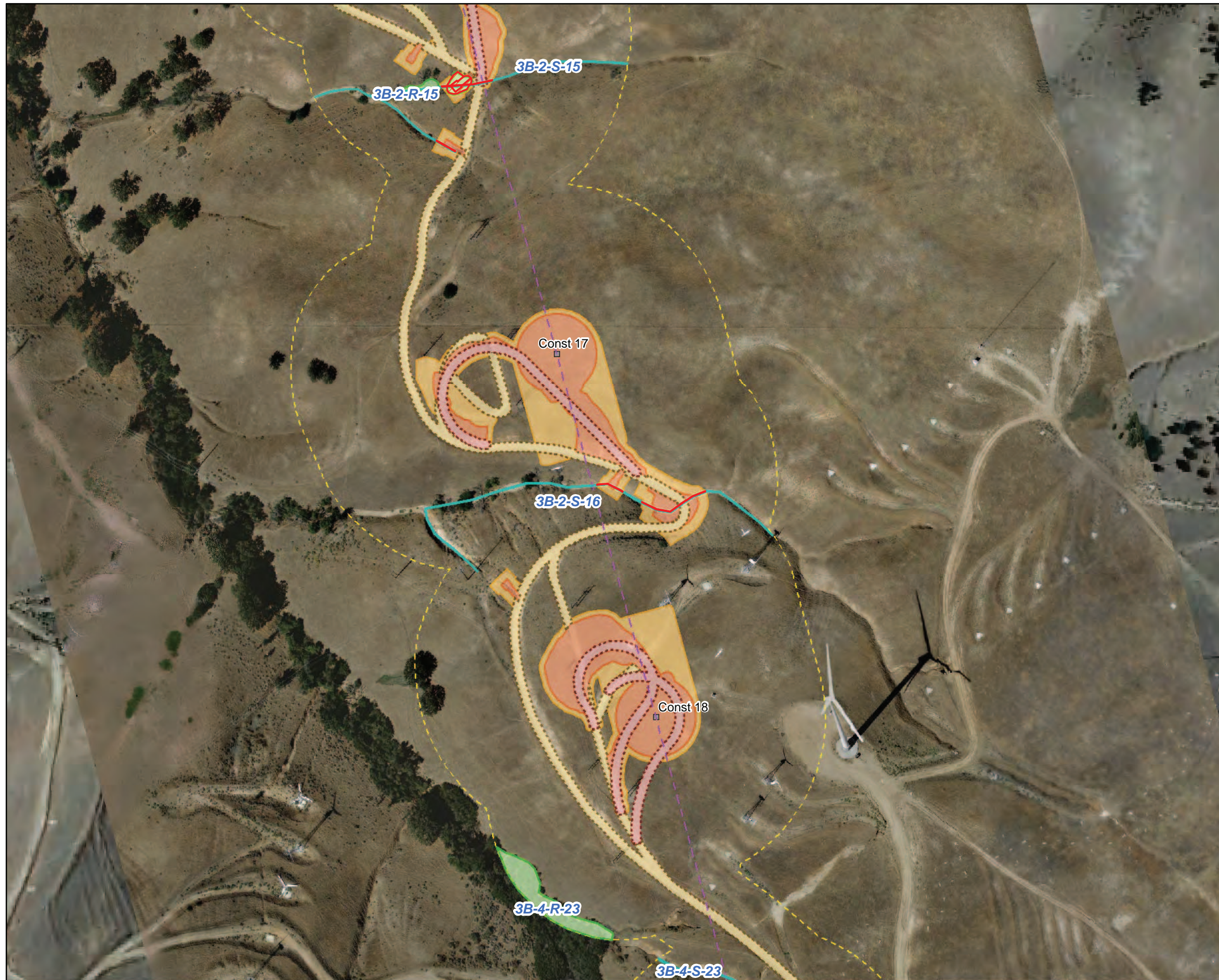
Figure 7 Representative Map of Impacts to Waters under the Water Board and CDFG Jurisdictions (Constructs 17 and 18 – New Access Road plus installation of two McCarthy drains, widening of existing access road, installation of new McCarthy drain and maintenance grading of existing access road) Attachment D Antelope Transmission Project – Segment 3B
