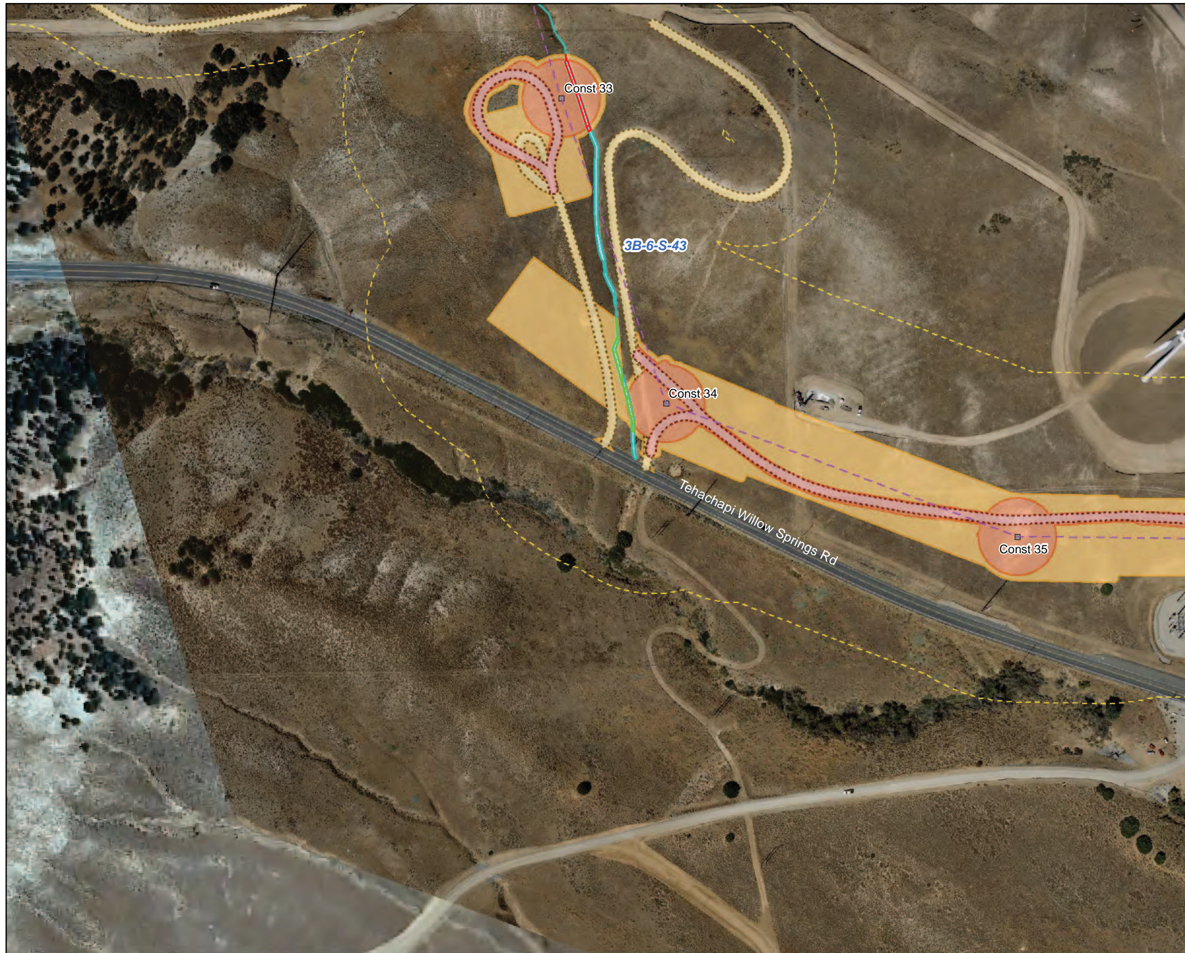
Figure 9 Representative Map of Impacts to Waters under the Water Board and CDFG Jurisdictions (Construct 33 – Construct 33 and permanent O&M area located within stream channel and will be converted to rip-rap lined channel for approximately 32 feet) Attachment D Antelope Transmission Project – Segment 3B
