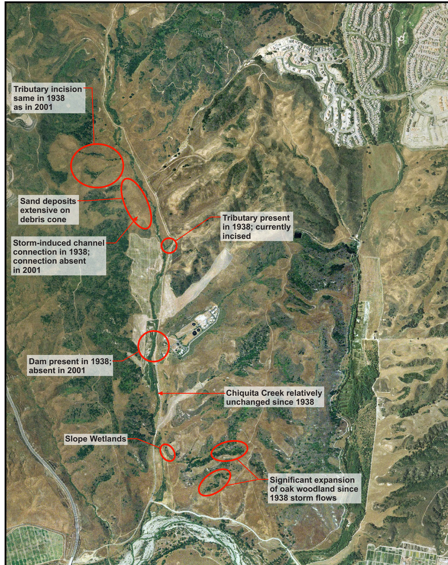
Figure 18 Lower Chiquita 1938 and 2001 Aerial Photographs
