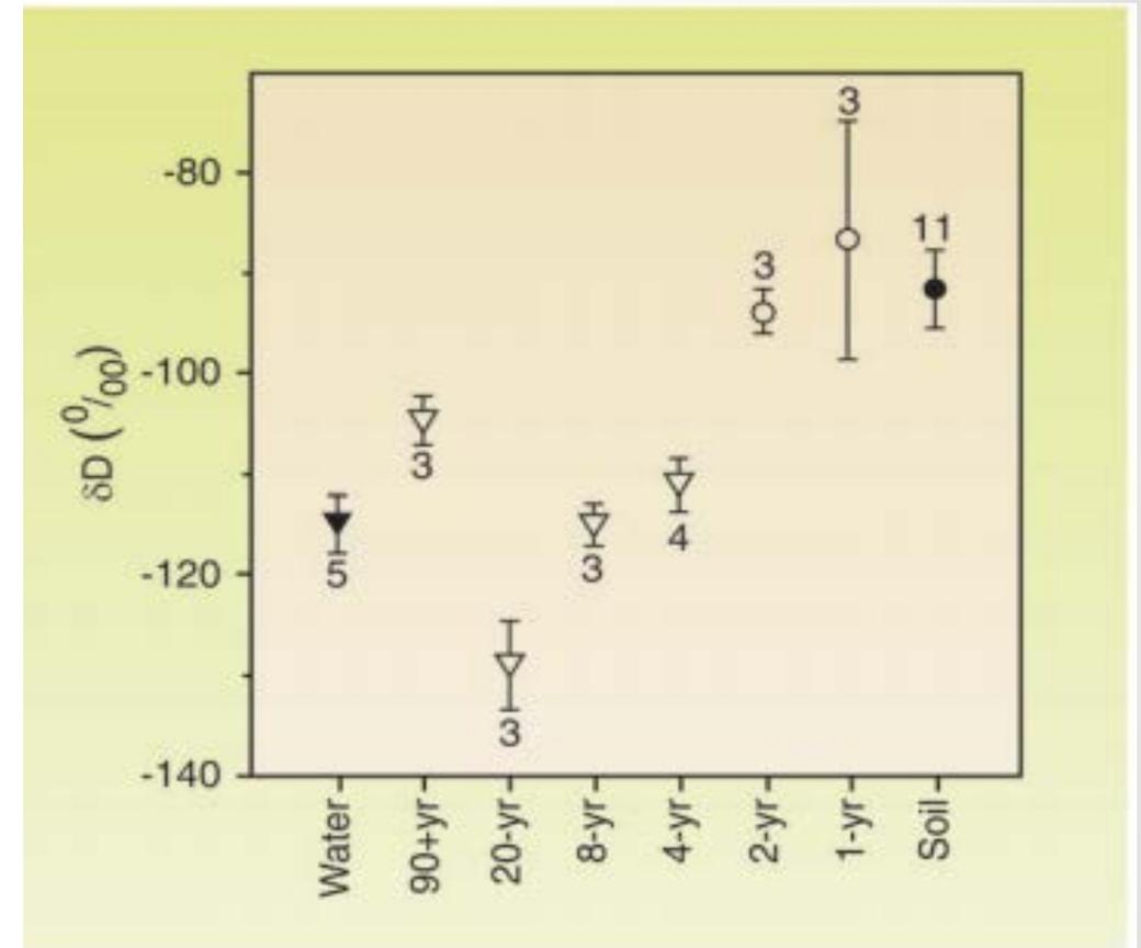
**Figure 3-7.** Sap water  $\delta D$  of groundwater (water); plants of 90+, 20-yr, 8-, 4-, 2-, and 1-year old cottonwoods; and soil water, illustrating that younger plants used primarily soil water.
