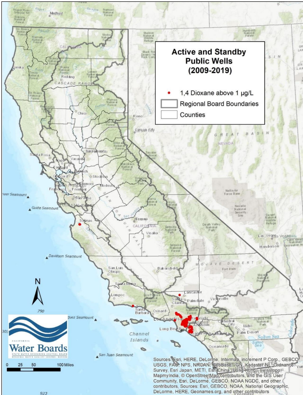
Figure 1. Active and standby public drinking water wells that had at least one detection of 1,4 Dioxane above the NL, 2009-2019, 194 wells. (Source: GAMA GIS )
