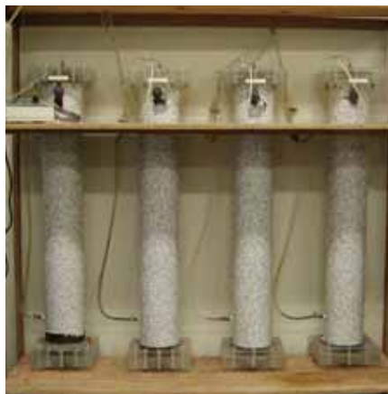
Figure 2.1. Soil-column system at CSM simulating anoxic, saturated flow conditions.
