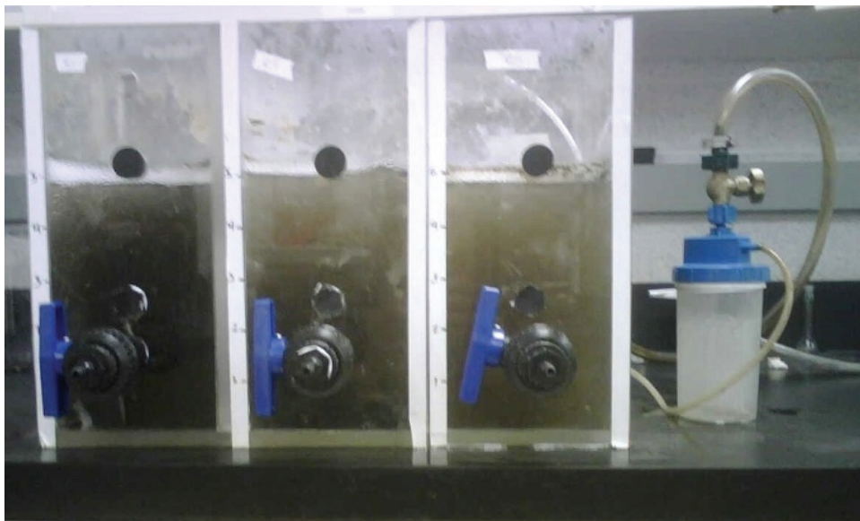
Figure 5.1. Experimental setup of the sequencing batch reactors. R1 is on the left, R2 in the middle, and R3 on the right.
