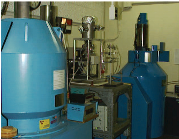
Figure 2.9. ^{60}\text{Co} sources housed at Notre Dame Radiation Laboratory.
