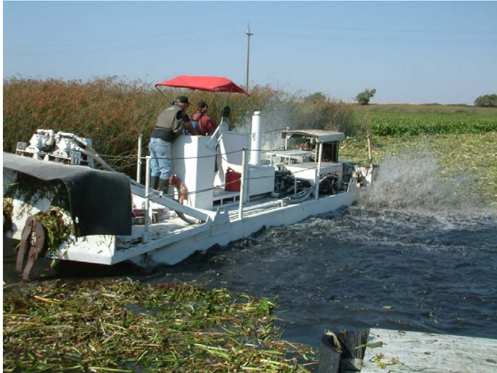
Figure 3. Mechanical shredding research pilot. Shredded hyacinth fragments are released into the water body
