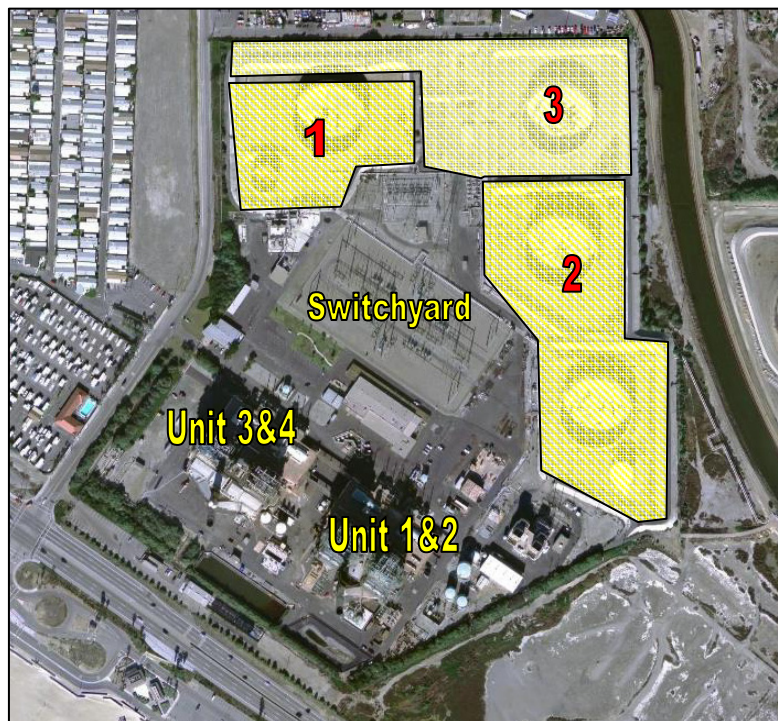
Figure G-3. Cooling Tower Siting Locations
