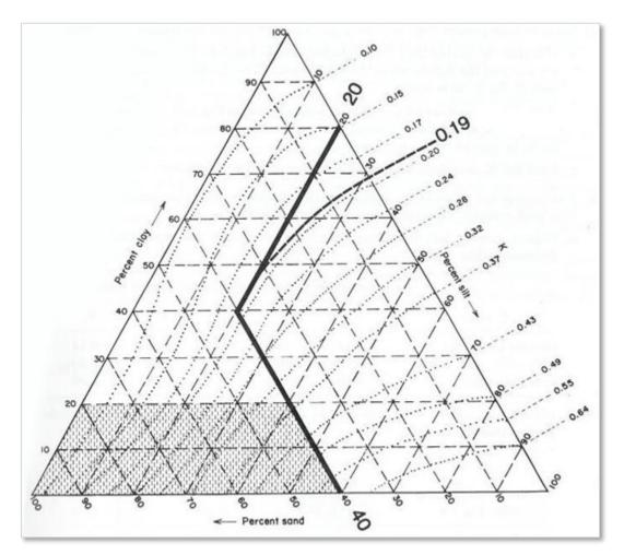
The figure above is the Erickson triangular nomograph used by the USDA to determine the K factor for a soil based on its texture (percent silt plus very fine sand, percent sand, percent organic matter, soil structure, and permeability).
