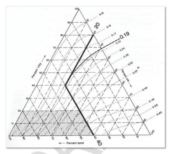
The K factor can be determined by using the nomograph method, which requires that a particle size analysis (ASTM D-422) be conducted to determine the percentages of sand, very fine sand, silt, and clay. Use the figure below to determine the appropriate K factor value.
