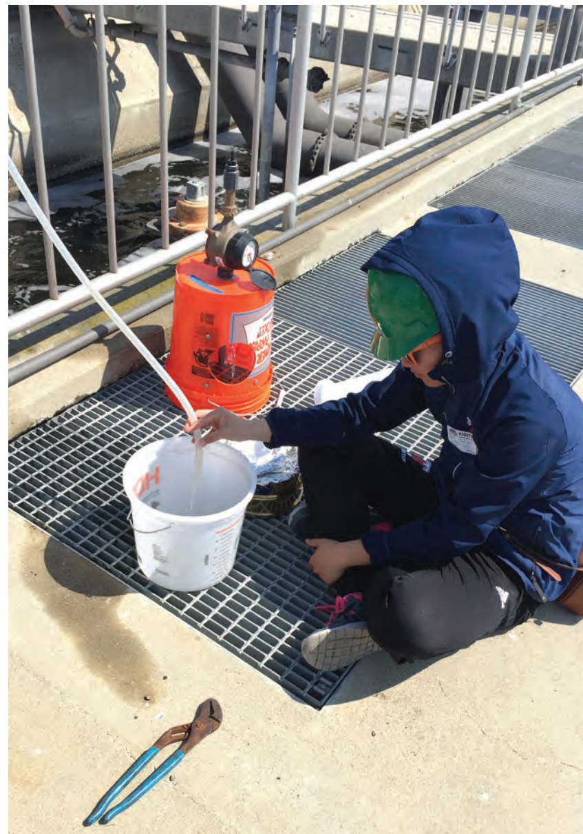
Sampling municipal wastewater for microplastic. Photograph by Meg Sedlak. >
