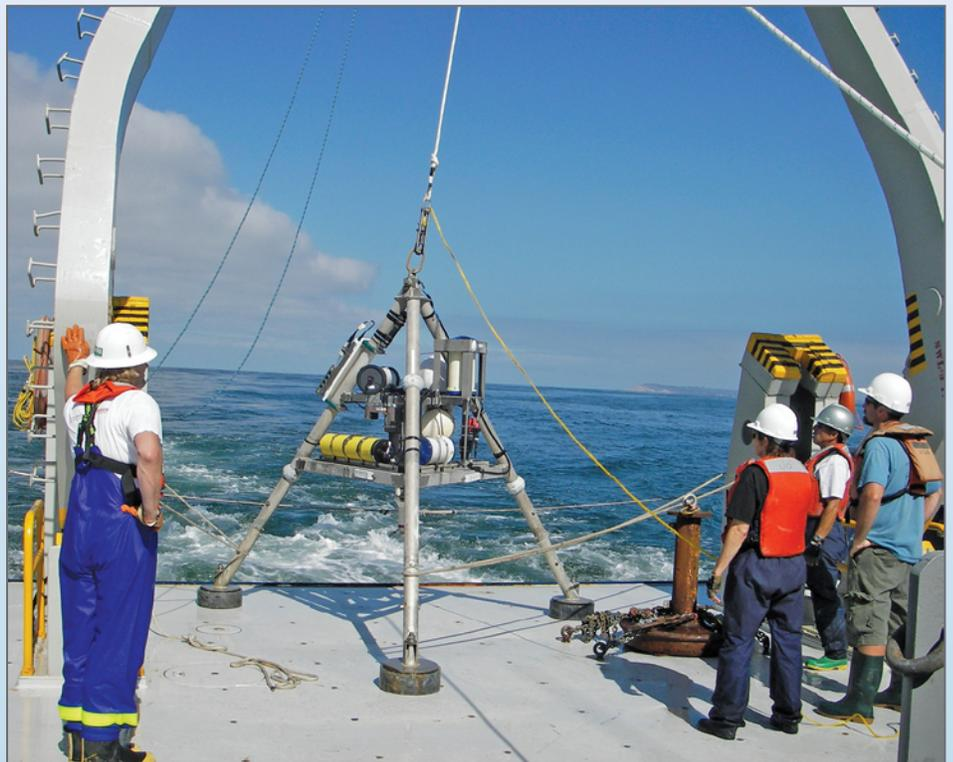
Above, scientists deploy a tripod with instruments to measure the effects of demonstration-project sediment and environmental conditions on ocean water turbidity.
