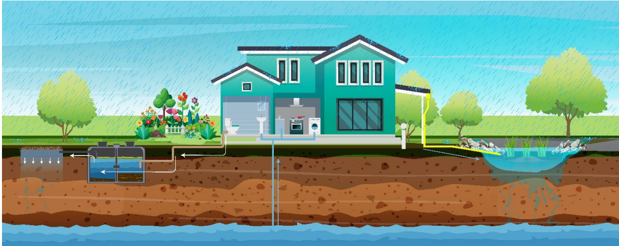
Figure 2 Figure showing a house with a septic system and domestic well on one side of the property. The infiltration system is on the other side of the house from the septic system and domestic well, at a safe distance from both.
