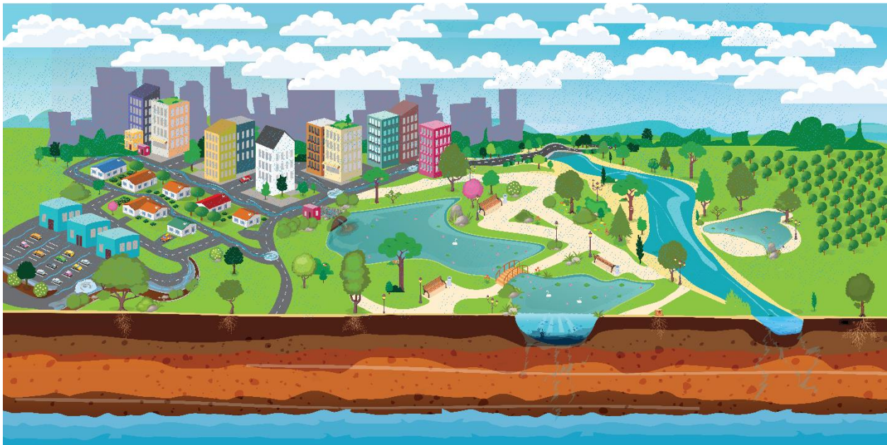
Figure 1: Rain runs off the city streets and into a storm drain, which drains into a nearby pond. The pond provides habitat for local wildlife and enables the stormwater to infiltrate into the ground and recharge the groundwater.
