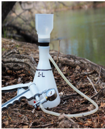
Figure 17. eDNA filtering options. Left: Hand-pump filtration units (cr. USGS). Right: vacuum manifold filtration set-up
