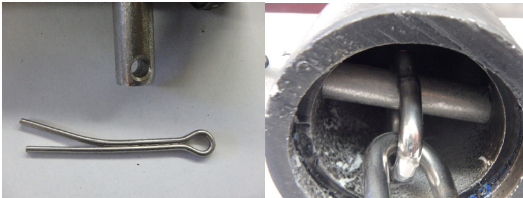
Figure 18. Clevis pin attachment to logger case, showing cotter pin (left) and chain link attachment to clevis pin (right).
