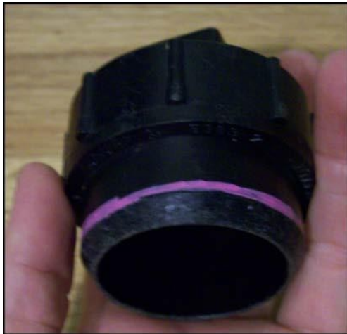
Figure 7. ABS delimiter, showing pink line at 1 cm depth mark. See Appendix A5 for assembly instructions.
