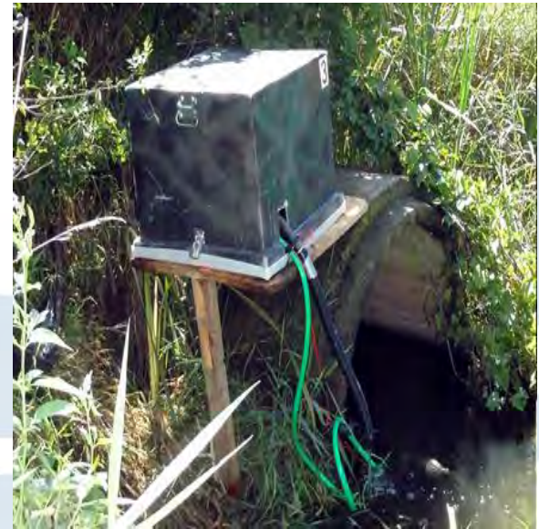
Self-contained battery-operated exposure unit placed on the bank of the river for field exposure of adult fathead minnows.
