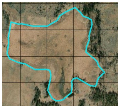
Figure 4.2: Examples of excluded and included waterbodies for custom shapefile construction. Santa Rosa Creek Reservoir was excluded as it does not contain a complete pixel, while Baseball Reservoir was excluded as it appeared to be dried up. Black squares indicate OLCI common grid pixels. Martha Lake was included in the inventory, while Santa Rosa Creek Reservoir and Baseball Reservoir were excluded from the inventory. True color basemap imagery courtesy of ArcGIS Pro World Imagery (Map Version 2023).
