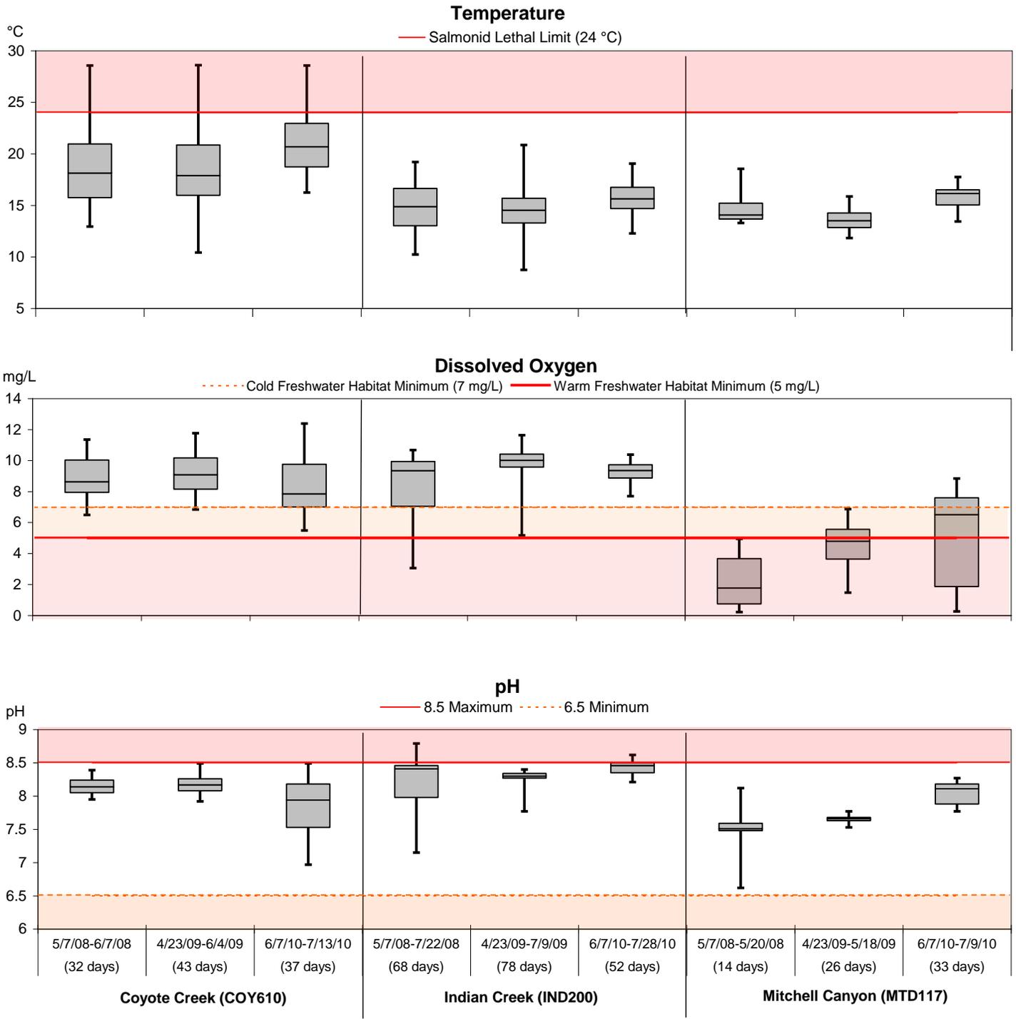
**Figure 3.6-2a: Summaries of time-series field measurements of temperature, dissolved oxygen, and pH in non-perennial reference sites in 2008-2010**
