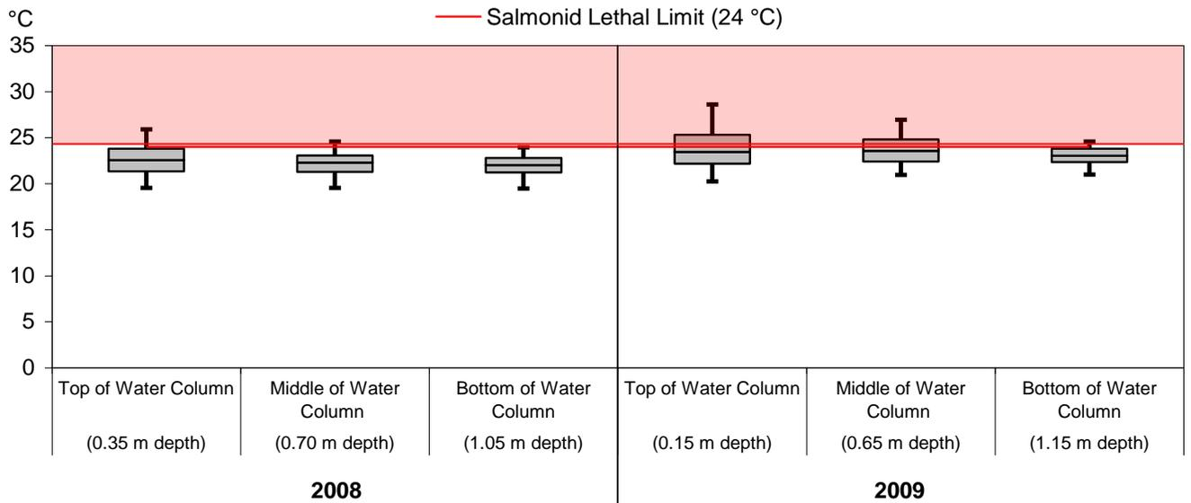
**Figure 3.6-4a: HOBO time-series field measurements along a vertical depth gradient at COY610 in 2008 and 2009**
