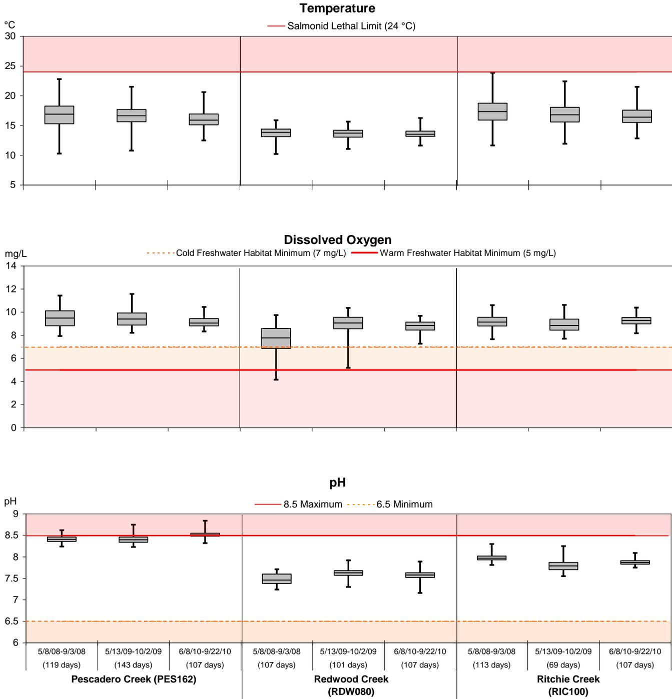
**Figure 3.6-2b: Summaries of time-series field measurements of temperature, dissolved oxygen, and pH in perennial reference sites in 2008-2010**
