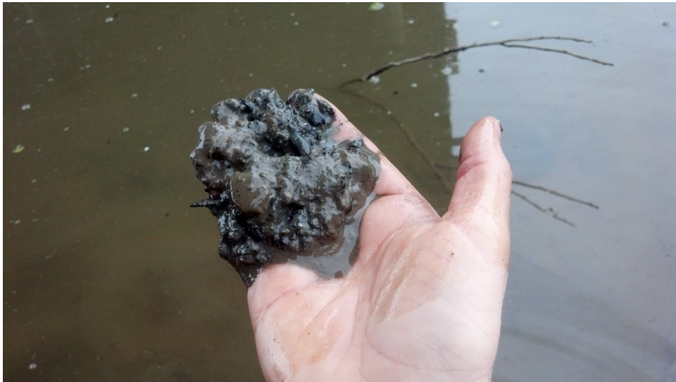
Figure 4.2.15. CBD channel sediment collected near the base of the east levee illustrating fine top layer over an organic rich mix of fine gravel to clay sediments.
