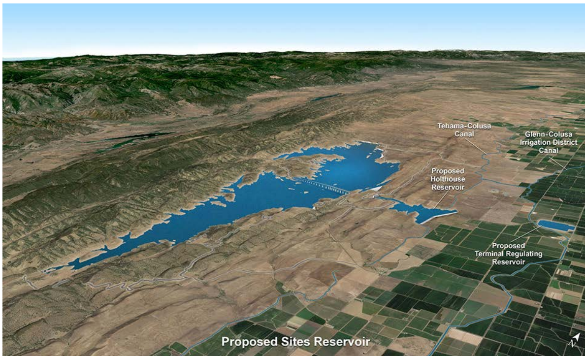
Figure 2.3.4. Artist's rendering of the latest proposed design for the NODOS, including the Sites, Holthouse, and Terminal Regulating Reservoirs (from DWR, 2014a).
