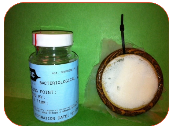
Figure 1. Photograph of a SPATT sampler next to a 4oz sample bottle.
