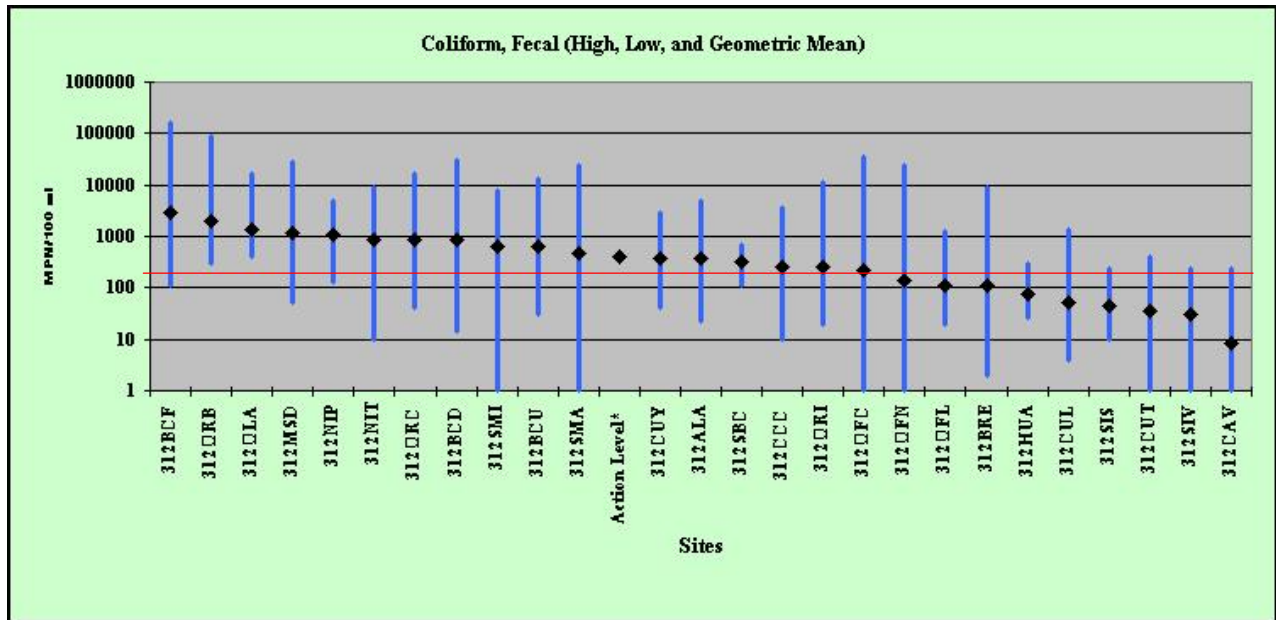
Figure 5.1.2b. Range and geometric mean of fecal coliform data collected monthly at sites in the Santa Maria Hydrologic Unit, January 2000 through March 2001. Red line corresponds to Basin Plan objective: geometric mean should not exceed 200 MPN/100mL.
