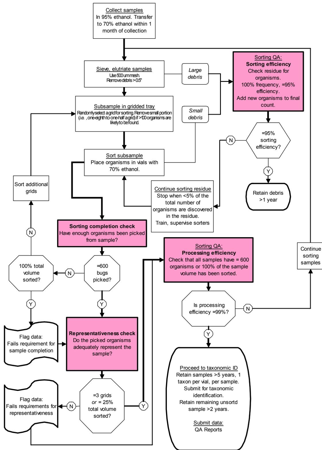
Figure 4B (Element 7). Sorting process diagram for sorting.
