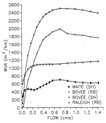
FIGURE 4.28.—Indices of suitable area (weighted usable area, WUA) versus flow (cubic meters per second) for juvenile steelhead (SH) and rainbow trout (RB) in a California atream based on different probability-of-use curves devised by Waite, Bovee, and Raleigh. (Inn Waite, unpublished data.)
