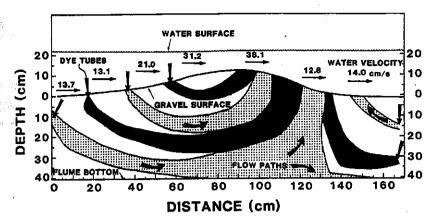
FIGURE 4.11.—Water flow through homogeneous gravel in a flume with a surface similar up that of a new salmon redd. Shadings indicate dispersions of injected dyes. (Redrawn from Cooper 1965.)
