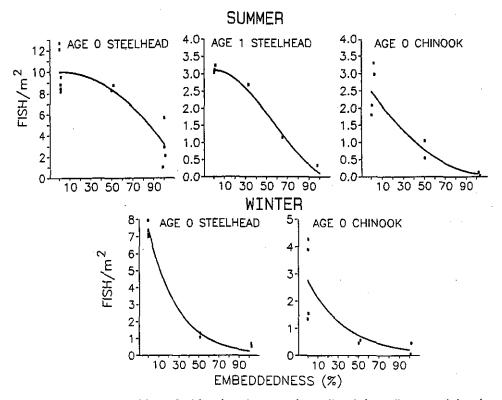
FIGURE 4.36.—Densities of chinook salmon and steelhead juveniles remaining in laboratory stream channels after 5 d during winter and summer tests to evaluate the effects of sedimentation. The channels had alternating pool-riffle configurations; fine sediments (<6 mm) were added to pools and riffles to embed the cobbles and boulders from 0 to 100%. (From Bjornn et al. 1977.)
