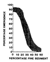
FIGURE 4.13.—Percentage emergence of swim-up fry placed in gravel-sand mixtures in relation to the percentage of sediment smaller than 2-6.4 mm in studies by Bjornn (1968), Phillips et al. (1975), Hausle and Coble (1976), and McCuddin (1977). The stipled area includes data from eight tests on brook trout, steelhead, and chinook and coho salmon.
