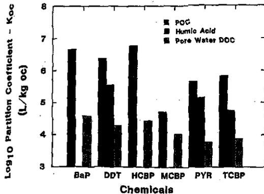
Fig. 13. Partition coefficients of chemicals to particulate organic carbon (POC), Aldrich humic acid, and natural DOC. Benzo[*a*]pyrene (BaP); 2,2',4,4',5,5' hexachlorobiphenyl (HCBP); DDT; 2,2',5,5'-tetrachlorobiphenyl (TCBP); pyrene (PYR); 4-monochlorobiphenyl (MCBP). Data from Eadie et al. [43].
