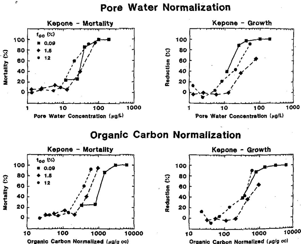
Fig. 21. Comparison of percent survival (left) and growth rate reduction (right) of *C. tentans* to Kepone concentration in pore water (top) and in bulk sediment, using organic carbon normalization (bottom) for three sediments with varying organic carbon concentrations [17].
