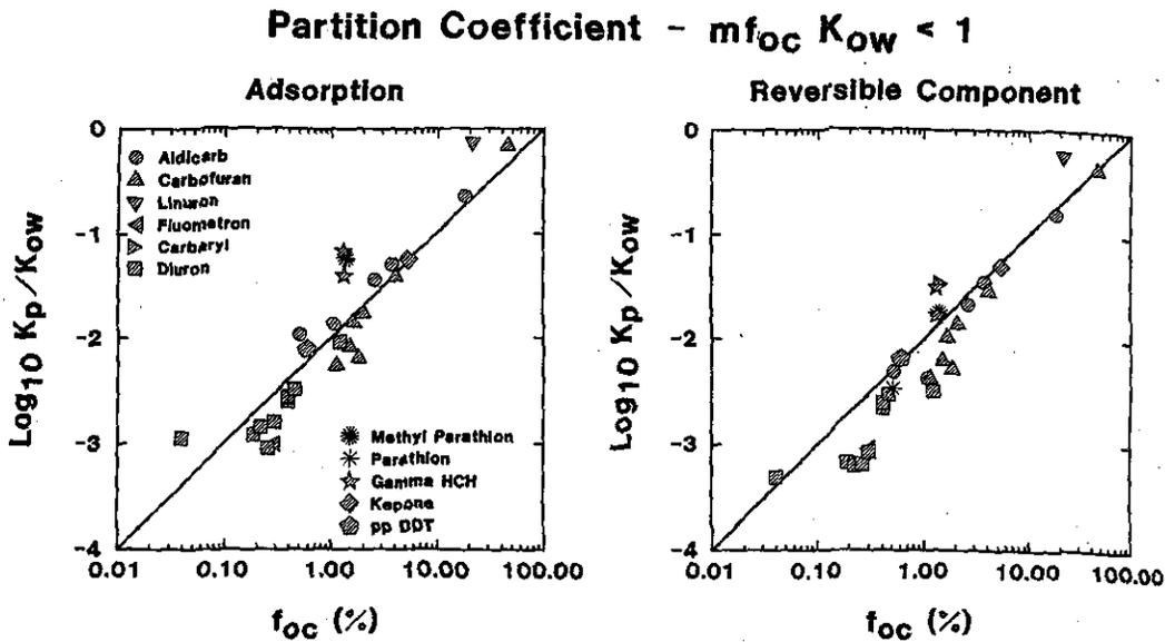
Fig. 12. Comparison of the normalized partition coefficients for adsorption (left) and reversible component sorption (right) to sediment organic carbon. The data are restricted so that particle effects are not expected to be significant:  $mf_{oc}K_{ow} < 1$ . The line represents perfect agreement [31].
