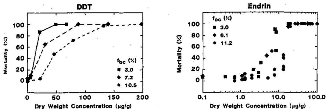
Fig. 7. Comparison of percent mortality of *H. azteca* to DDT (left) and endrin (right) concentrations in bulk sediment (top) and pore water (bottom) for sediments with varying organic carbon concentrations [21,22].
