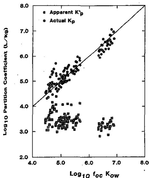
Fig. 19. Observed partition coefficient versus the product of organic carbon fraction and octanol/water partition coefficient. The line represents equality. The partition coefficients are computed by using total dissolved PCB (squares), and free PCB (circles) which is computed with Equation 26 with  $K_{DOC} = K_{ow}$ . Data from [50].
