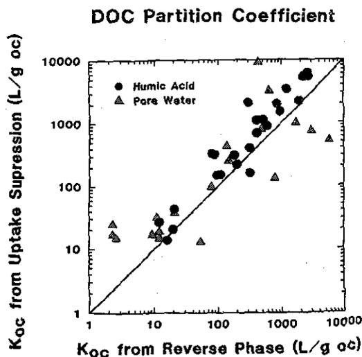
Fig. 16. Comparison of the DOC partition coefficient calculated from the suppression of chemical uptake versus the  $C_{18}$  reversed-phase HPLC column estimate. Circles are Aldrich humic acid; triangles are interstitial water DOC. Chemicals are listed in Figure 15 caption (also anthracene and benzo[a]anthracene).
