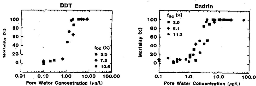
Fig. 22. Comparison of percent survival of *H. azteca* to DDT (left) and endrin (right) concentration in pore water (top) and in bulk sediment, using organic carbon normalization (bottom) for three sediments with varying organic carbon concentrations [21,22].
