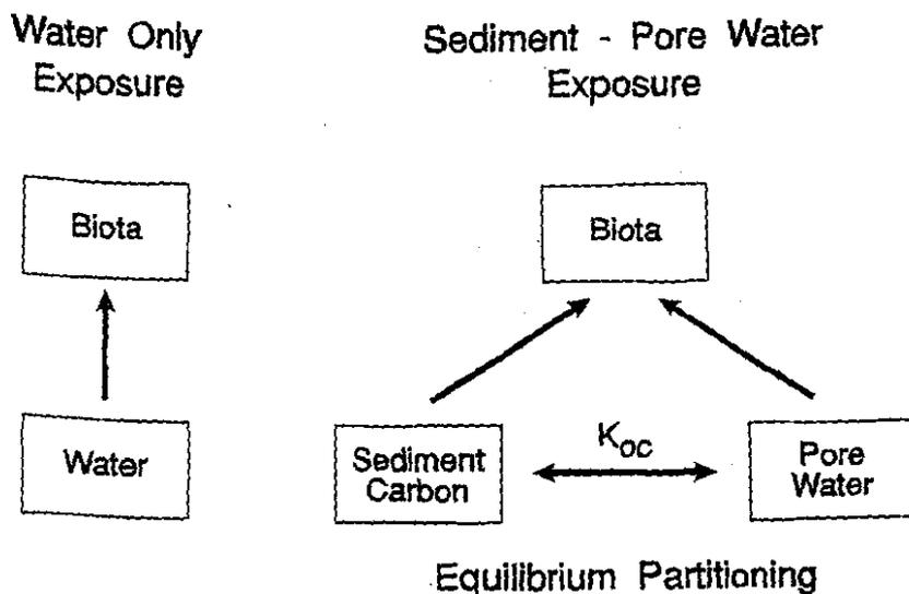
Fig. 1. Diagram of the organism exposure routes for a water-only exposure (left) and a sediment exposure (right). *Equilibrium partitioning* refers to the assumption that an equilibrium exists between the chemical sorbed to the particulate sediment organic carbon and the pore water. The partition coefficient is  $K_{oc}$ .
