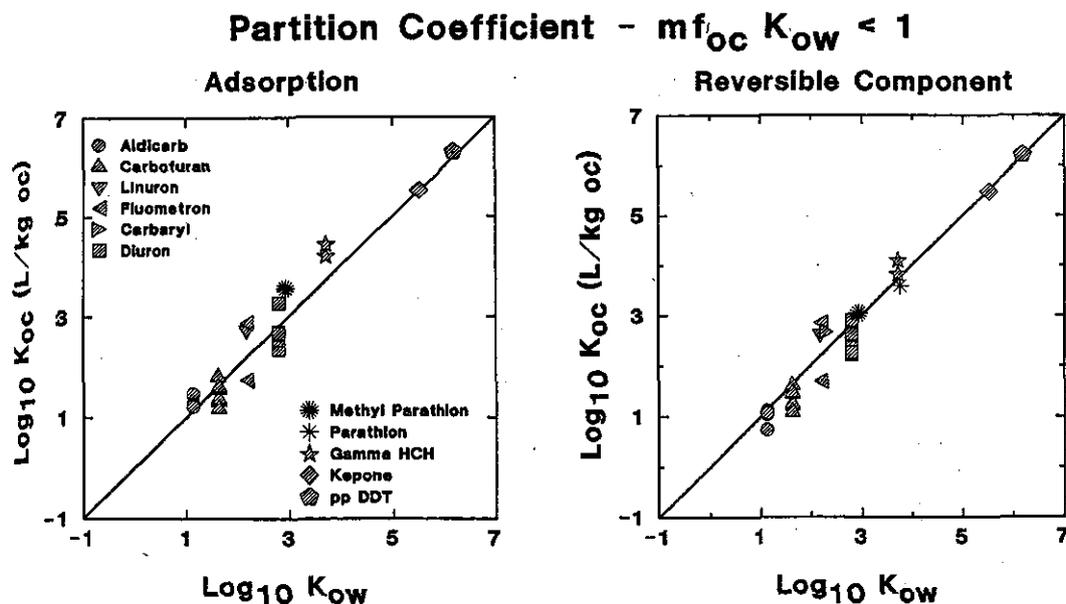
Fig. 11. Comparison of the adsorption (left) and reversible component (right) organic carbon-normalized partition coefficient,  $K_{oc}$ , to the octanol/water partition coefficient,  $K_{ow}$ , for experiments with low solids concentrations:  $mf_{oc}K_{ow} < 1$ . The line represents equality [31].
