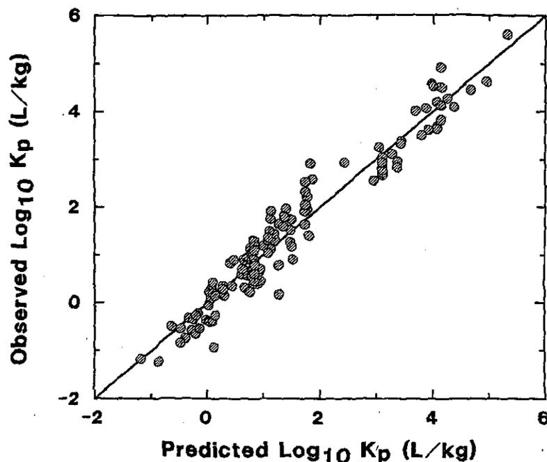
Fig. 10. Comparison of observed reversible component partition coefficient to calculated partition coefficient using Equation 10 [31].
