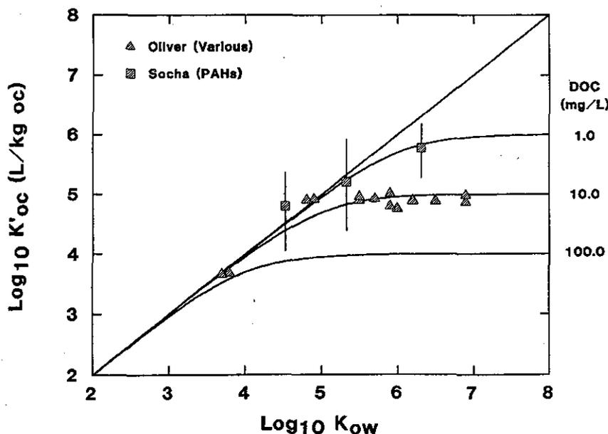
Fig. 20. Observed apparent partition coefficient to organic carbon versus the octanol/water partition coefficient. The lines represent the expected relationship for DOC concentrations of 0, 1, 10, and 100 mg/L and  $K_{DOC} = K_{ow}$ . Data from [53] for PCB congeners and other chemicals and from [52] for phenanthrene, fluoranthene, and perylene.
