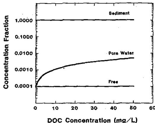
Fig. 14. Phase distribution of a chemical in the three-phase system: water, sediment, and DOC (Eqns. 18, 19, and 20).  $K_{oc} = K_{DOC} = K_{ow} = 10^6$  L/kg,  $f_{oc} = 2.0\%$ , and  $m = 0.5$  kg/L.
