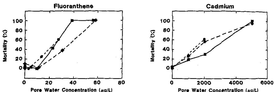
Fig. 6. Comparison of percent mortality of *R. abronius* to fluoranthene [19] (left) and cadmium [20] (right) concentrations in bulk sediment (top) and pore water (bottom) for sediments with varying organic carbon concentrations.
