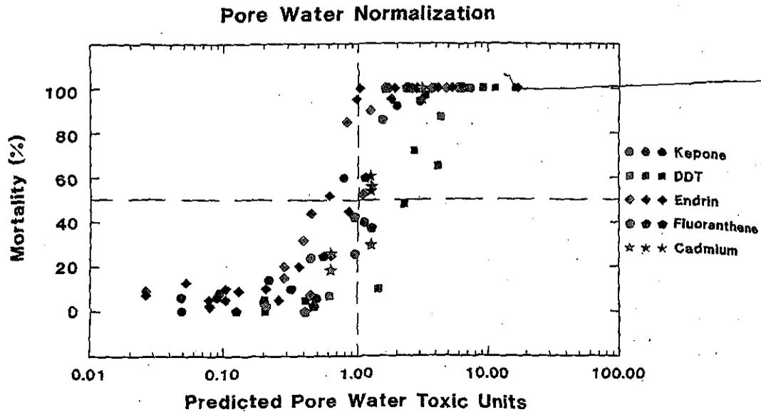
Fig. 2. Mortality versus predicted pore water toxic units for five chemicals and three sediments per chemical. Sediment types are indicated by the single hatching (lowest organic carbon content), cross-hatching (intermediate organic carbon content), and filled symbols (highest organic carbon content). See Tables 1 and 2 for data sources. Predicted pore water toxic units are the ratio of the pore water concentration to the water-only LC50 (Eqn. 1).
