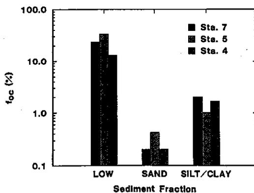
Fig. 17. The organic carbon fractions (% dry weight) in the low-density fraction  $>64 \mu\text{m}$ ,  $<1.9 \text{ g/cm}^3$ ; the sand-sized fraction  $>64 \mu\text{m}$ ,  $>1.9 \text{ g/cm}^3$ ; the silt/clay-sized fraction  $<64 \mu\text{m}$ . Numbered stations as indicated. Data from Prahl [48].
