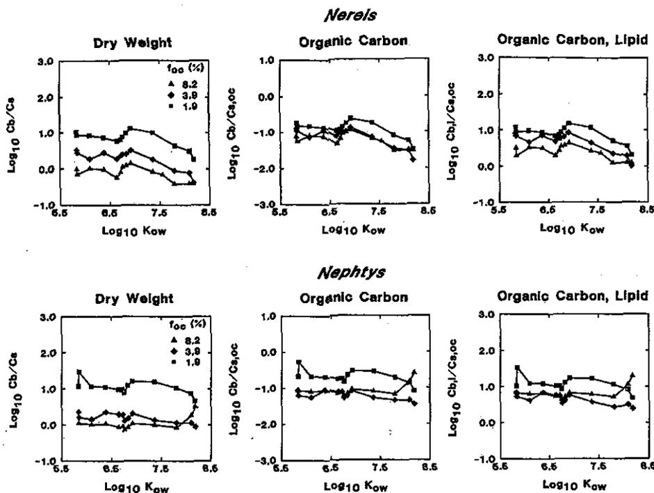
Fig. 24. Plots of the BSF (ratio of organism-to-sediment concentration) for three sediments for a series of PCB congeners versus the  $\log_{10} K_{ow}$  for that congener. The dry weight normalization for both organism and sediment (left panels); organic carbon normalization for the sediment (middle panels); and organic carbon and lipid normalization (right panels) as indicated. The organisms are *Nereis* (top) and *Nephtys* (bottom). Data from [58].
