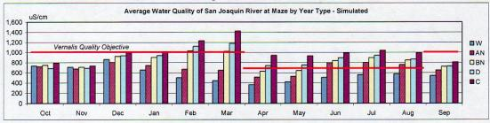
Figure 6: CALSIM II-Revised simulation of San Joaquin River Electrical Conductivity at Vernalis. (Periodic Review SJRG-13, p20.)
