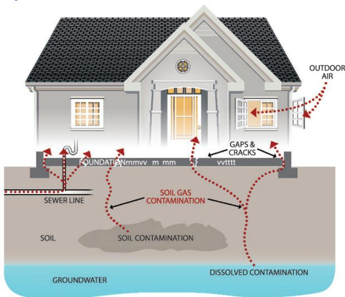
Inhalation of harmful vapors from contamination off-gassing is a significant health hazard. These vapors are often
