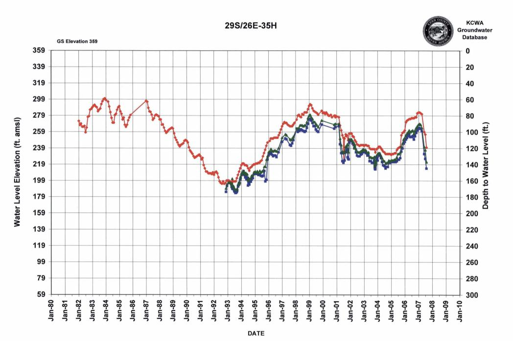
PERF INTERVAL 300'-500' (Shop) ——PERF INTERVAL 590'-680' ——PERF INTERVAL 310'-410'
